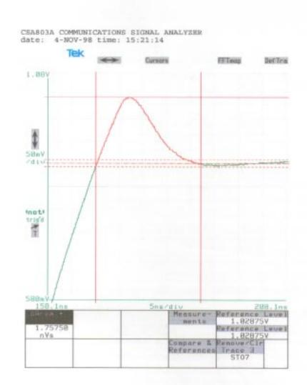
Figure 3 - CS803A Glitch Waveform
