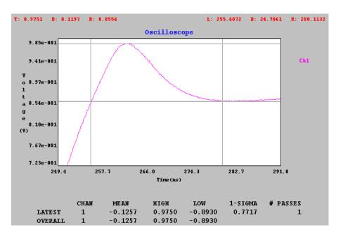
Figure 4 - Glitch Waveform Taken with VI Oscilloscope
